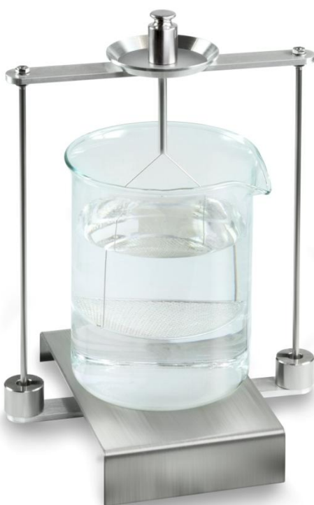
Fig. 1: Weighing in air
