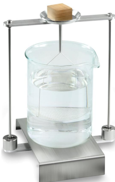
Fig. 3: Weighing in air
