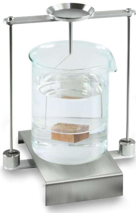
Fig. 4: Weighing in auxiliary liquid
