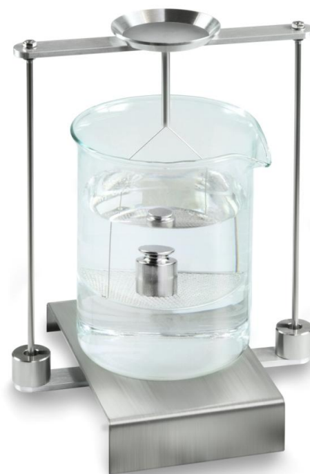
Fig. 6: Weighing in test liquid
